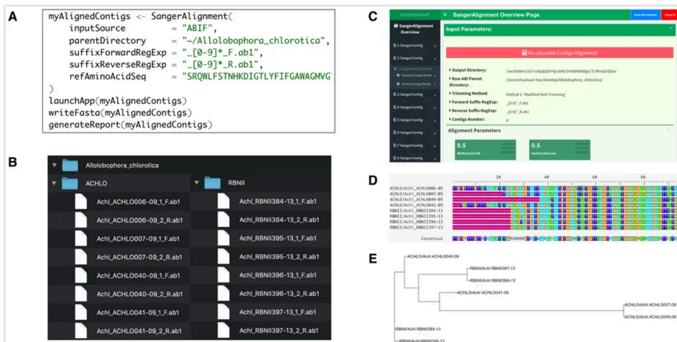
Figure 2. A complete analysis of eight samples. (A) The few lines of R that drive it. (B) The ABIF input files, organized in folders and named so the package can infer contig groups and read direction. (C) The optional Shiny overview page. (D) The resulting multiple sequence alignment of the eight consensus contigs, and (E) a tree used as a quality-control view.
